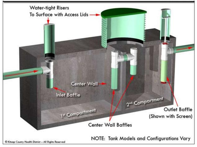
**NOTE:** The effluent screen in the outlet baffle is optional.
